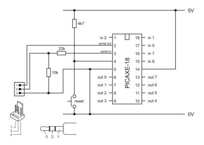
The 4k7 resistor is used to pull the PICAXE microcontrollers reset pin (pin 4) high. If desired, a reset switch can also be connected between the reset pin (pin 4) and 0V. When the switch is pushed the PICAXE microcontroller 'resets' to the first line in the program.
