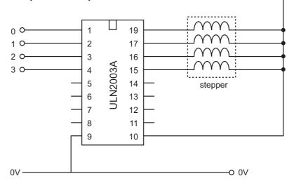
To make the armature rotate continuously the four coils inside the stepper motor must be switched on and off in a certain step order. The ULN2003A driver chip on the tutorial board provides the method of interfacing these four coils.
