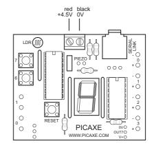
circuit board, or a pre-made interface or tutorial board may be used for speed and convenience. This course presumes use of a PICAXE-18M2 (18 pin) microcontroller mounted on the tutorial board.
