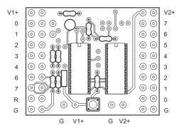
This is a project board that provides 8 digital (on/off) outputs via a darlington driver IC.
