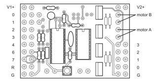
This is a project that provides 4 digital outputs (via FET drivers) and 2 reversible motor outputs.
