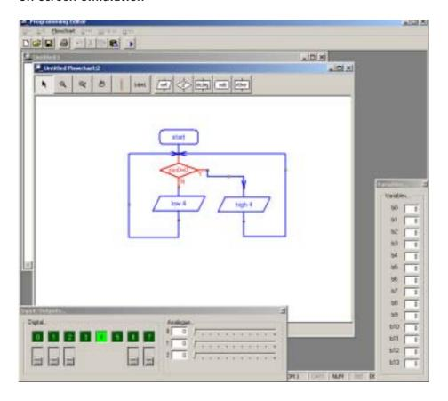
To simulate the flowchart, click 'Simulate' from the Flowchart menu. The program will then start to run on-screen.
