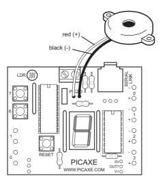
The PICAXE system can automatically create noises of different frequencies by use of the sound command.
