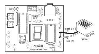
Buzzers will make a noise when they are connected to a power supply. This noise is usually 'fixed' at one frequency and so buzzers can only make one 'tone'. Piezo-sounders use a different type of system to create noises, and can be used to create noises of different tones by providing them with a 'pulsed' output.
