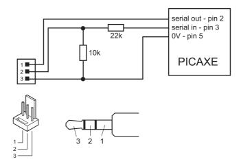
It is strongly recommended that this interfacing circuit is included on every PCB designed to be used with the PICAXE microcontroller. This enables the PICAXE microcontroller to be re-programmed without removing from the PCB.
