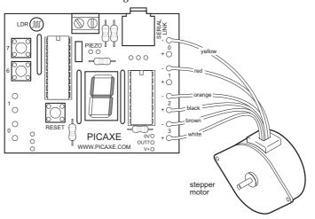
The stepper motor should be connected to the holes on the tutorial board as follows:
