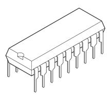
The 'brain' of the PICAXE system is the 18 pin PICAXE18M2 microcontroller. Although microcontrollers are relatively cheap (some microcontrollers cost less than £1) microcontrollers are very complex devices containing many thousands of transistors, resistors and other electronic components.
