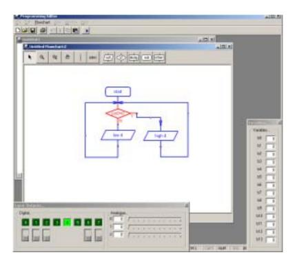
The Flowchart Editor allows flowcharts to be drawn and simulated on-screen. The flowchart can then be automatically converted into a BASIC program for downloading into the microcontroller.
