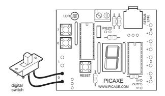
This program below shows how to react to switch pushes . In this program output pin 7 flashes every time the push switch on input pin 6 is pushed.
