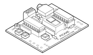
The 'PICAXE' system is an easy-to-program microcontroller system that uses a simple BASIC language, which most students can learn very quickly. The PICAXE system exploits the unique characteristics of the new generation of low-cost 'FLASH' memory based microcontrollers. These microcontrollers can be programmed over and over again without the need for an expensive PIC programmer.
