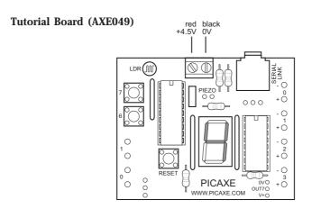
This is a tutorial board containing switches, sensors, a seven segment display and output drivers. This is the board described in these notes.
